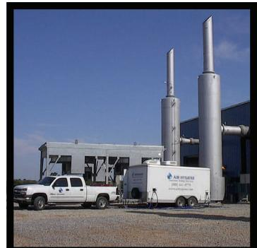
For most 4J testing the scope is 3, 1-hour test runs monitoring for NO<sub>x</sub>, CO, VOCs, and O<sub>2</sub>. The VOC analysis methodology described in Table 2 of the regulation calls for:
